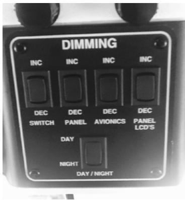
An overhead-light control panel, easily accessible to the pilot incorporates a functional arrangement of all lighting systems in the cockpit. Each light group has its own back-lit rheostat which allows for dimming of the cockpit lights. These switches control the panel lights, radio panel lights, and EFIS instrument lights. The overhead cockpit ceiling lights are individually controlled by separate switches.
